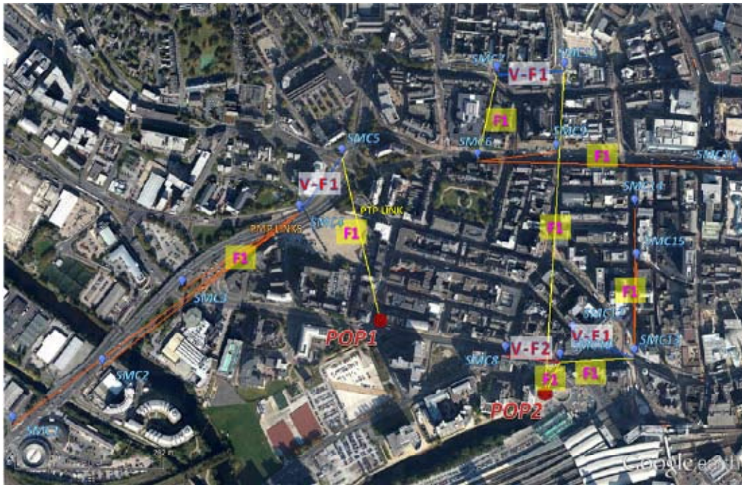
Figure 2: Distribution of Small Cells in a European city (shown in blue) and the links used for their backhauling. PtP MW links are shown in yellow and PtMP MW links in orange (all use the same 56 MHz channel denoted as F1 in yellow background). The 60 GHz links are shown as lines in Blue (channel V-F1) and Red (channel V-F2).
